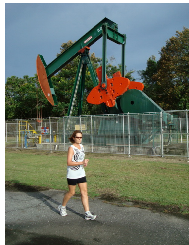
3 Rod pump behind Brunei Shell Head Office
